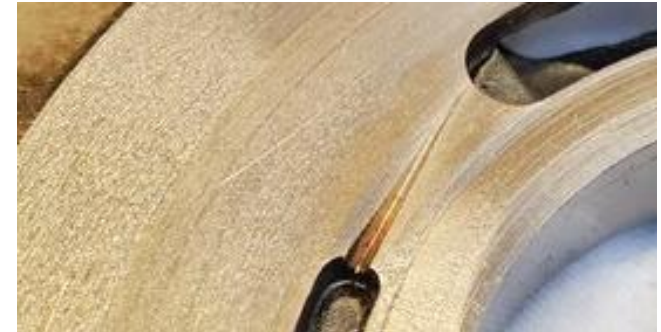
✓ Teardown showing abrasive wear
